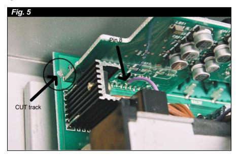
Connect the purple wire onto the connector CY142 pin 8.
